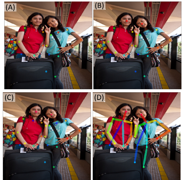
Figure 5. Body part parsing: (A) Estimated high joint location, (B) Estimated low joint location, (C) Both Joints after body part parsing, (D) Skeleton output after individual parsing
